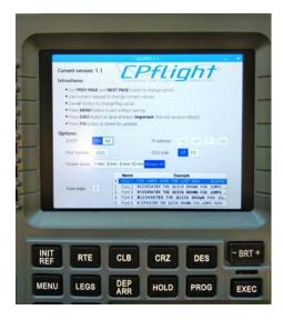
In this window you can see the assigned ip address ( useful for example to configure Prosim window ), and other option to customize your CDU. In the upper side of the monitor a legend will drive you to use the buttons to browse into MENU' window.
