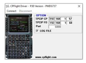
Run Prepar3d and load a PMDG flight. From CPflight folder run the application CDU\_COM.exe and select "Connect" into CDU\_COM application menu bar.
